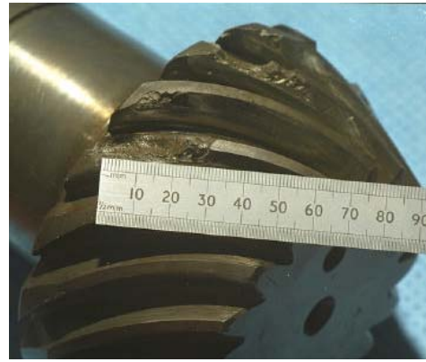
Damaged input bevel gear teeth.
